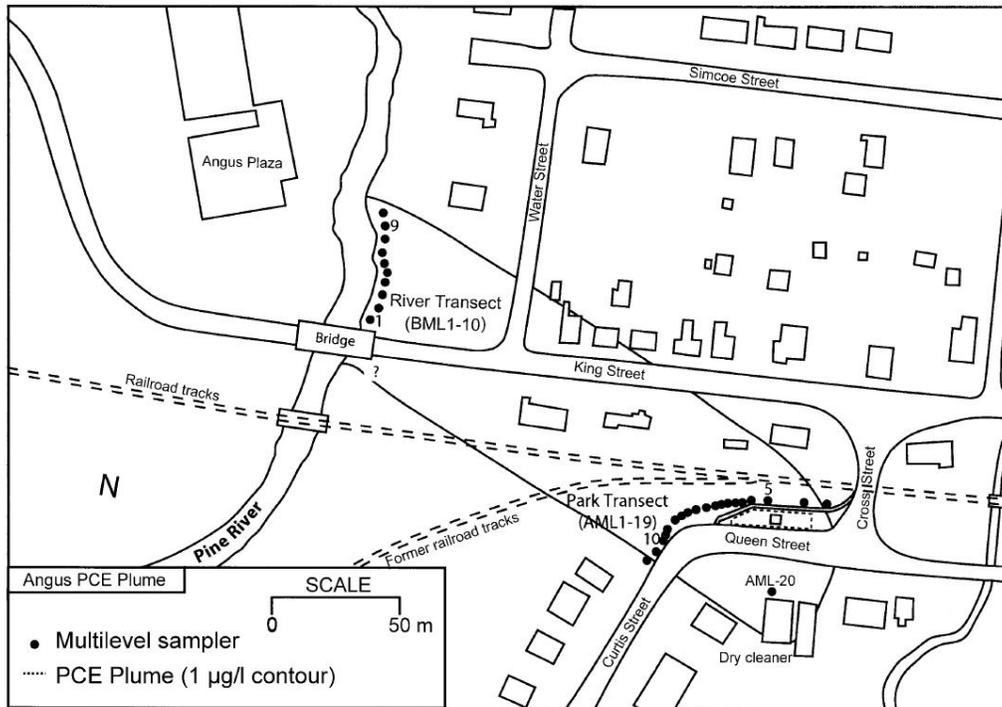
**Figure 8.** Dry Cleaner Site, Angus Field, showing multilevel sampler locations. (Hunkeler, et. al.)
