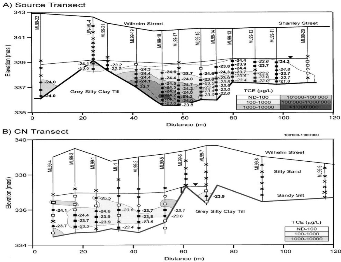
Figure 6. Cross-sections of the Kitchener TCE Plume. (Hunkeler, et. al.)
