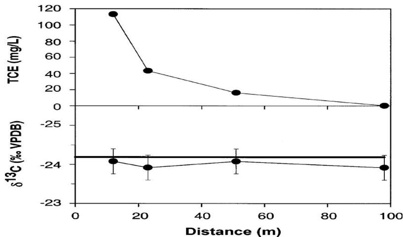
Figure 7. TCE concentration and δ<sup>13</sup>C of TCE for sampling point with highest TCE concentration in ML99-19, ML-3P, ML-2P, and ML99-7 as a function of distance from source at the Kitchener site. (Hunkeler, et. al.)
