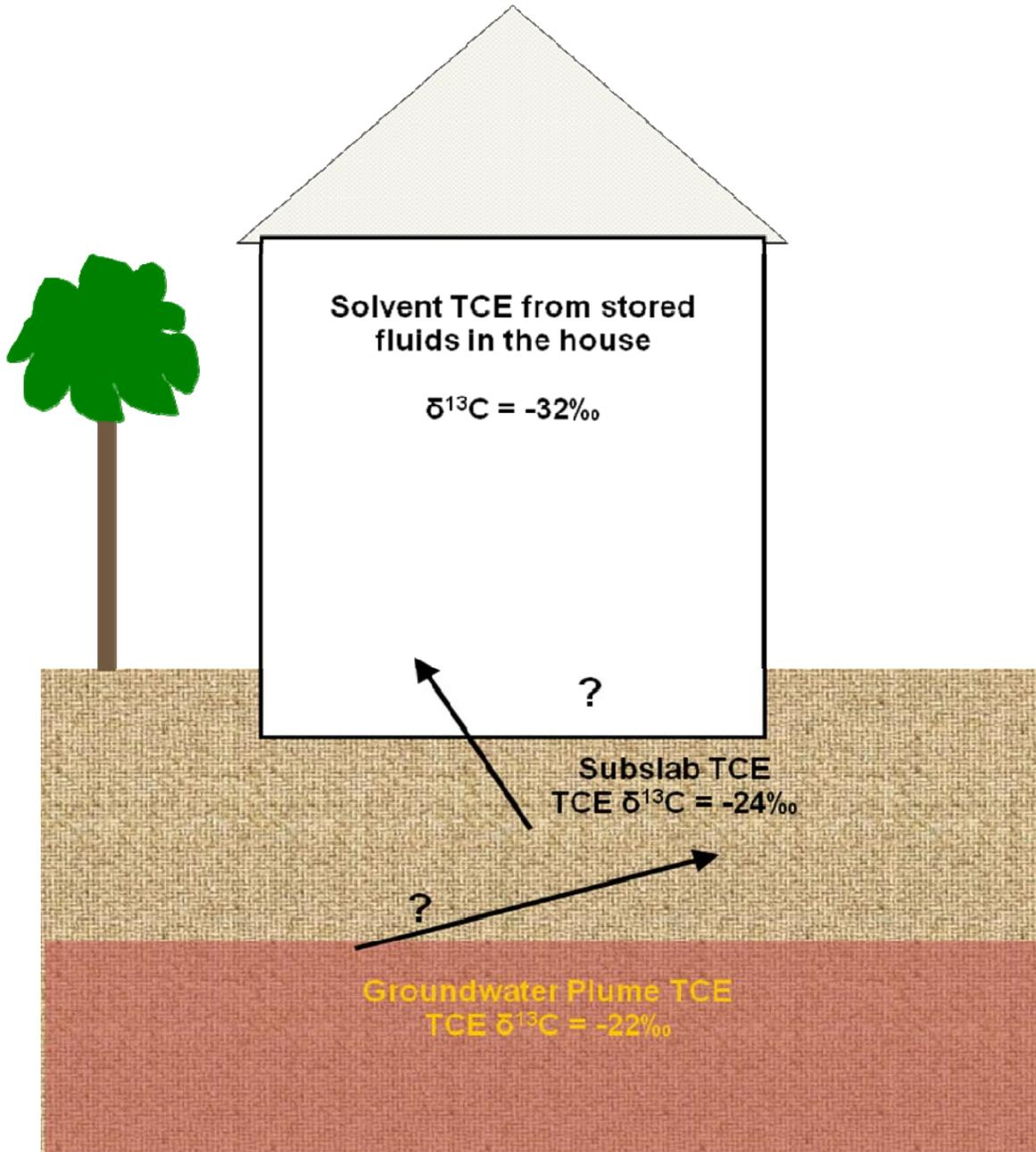
**Figure 15.** Application of CSIA to Vapor Intrusion (Burns, et.al.)
